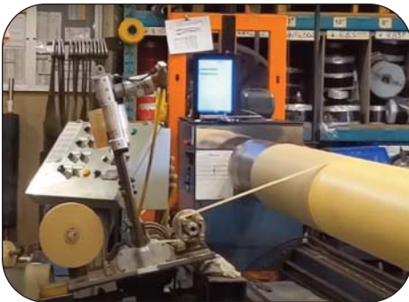
Automated winding cover application process
