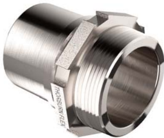
Style 73MBSPT | Male BSPT Fitting - Smooth Stem EN 14420-5/DIN 2817
