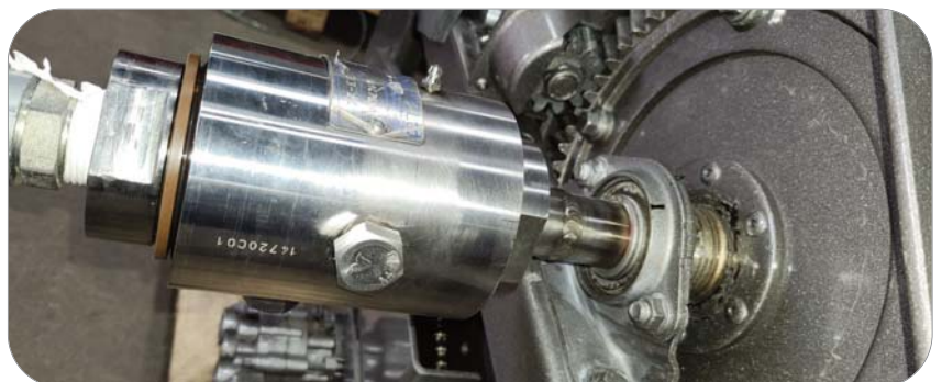
All wetted parts made from Duplex 2205 material including piping and live swivel joint
