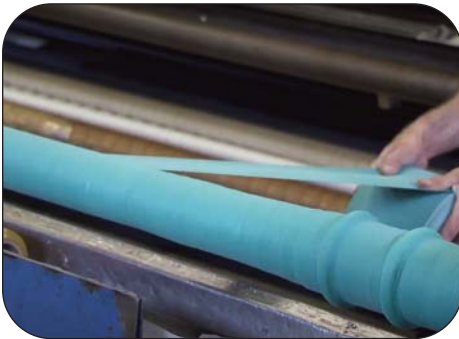
Hose tube layer winding process
