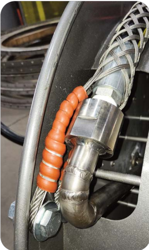
Whip Check added for safety
