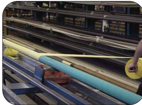
Fabric reinforcement winding process
